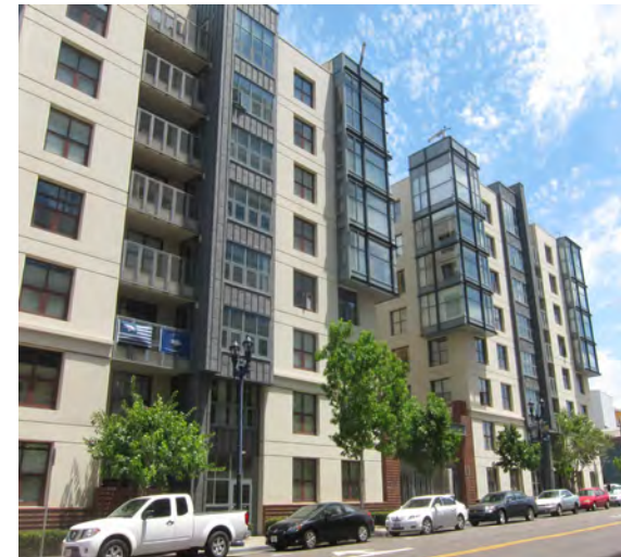
Use windows, walls, materiality and colours to articulate building facades so as to create fine-grain street frontages. Articulate the building form with set-backs or insets to help reduce the impact of building bulk on adjacent sidewalks.
