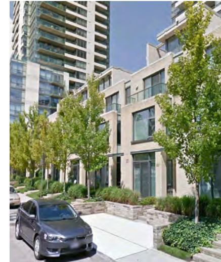
Provide grade separation and greater landscape setbacks between the sidewalk and ground floor of residential units to increase privacy for residents.
