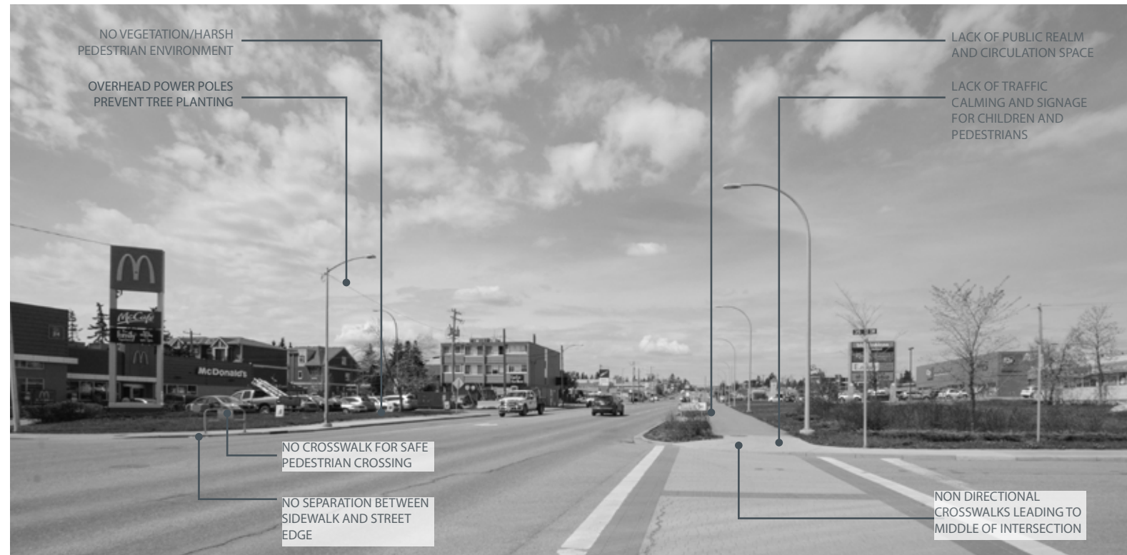
Figure 3.5 Existing Condition at Northwest Corner (17th Ave. and 35th St.)
