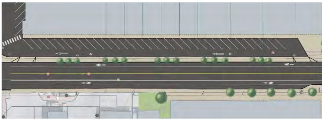
Angled parking closest to building face with driving lane behind
