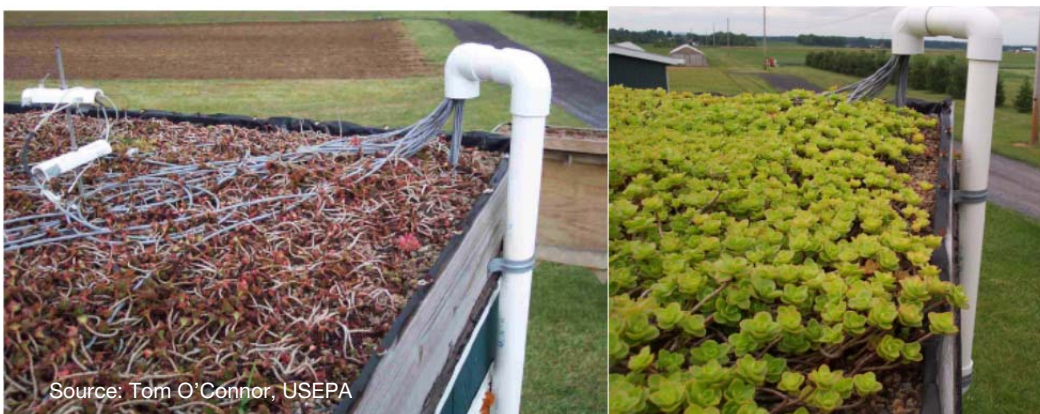
Figure 2. Example of monitoring equipment for a Green Roof.
